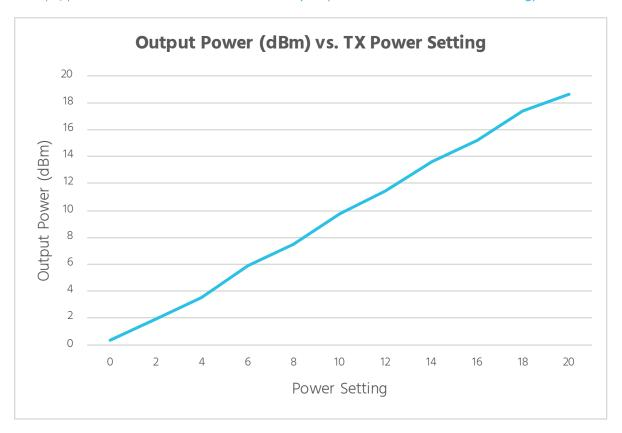
**Note:** The graph above is for the PA10 variant. For the PA11 module, the maximum output power is limited to 10.5 dBm.
